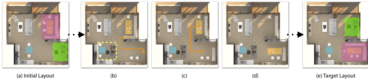
Fig. 9. “Smart moves” performed by Scene Mover in the living room example. (a) Initial layout. (b) To make way for the dining table to reach its target position, Scene Mover moved the obstacles, highlighted by a yellow dashed bounding box, to the lower-left corner, and then moved the bench to the lower-right corner. (c) Scene Mover moved the dining table to its target position. (d) Layout after moving the dining table. (e) Target layout. The areas to be swapped are high-lighted by the pink and green box in (a) and (e).
